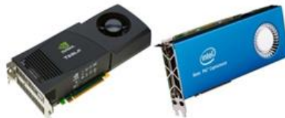
Accelerators / Coprocessors high compute density, high performance/watt
