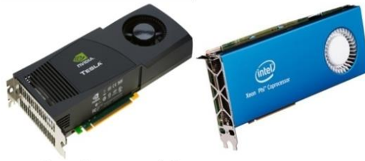
Accelerators / Coprocessors high compute density, high performance/watt
